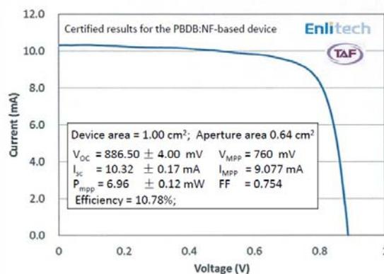
**Figure 1.** Photovoltaic properties of the PBDB-NF-based fullerene-free device.
