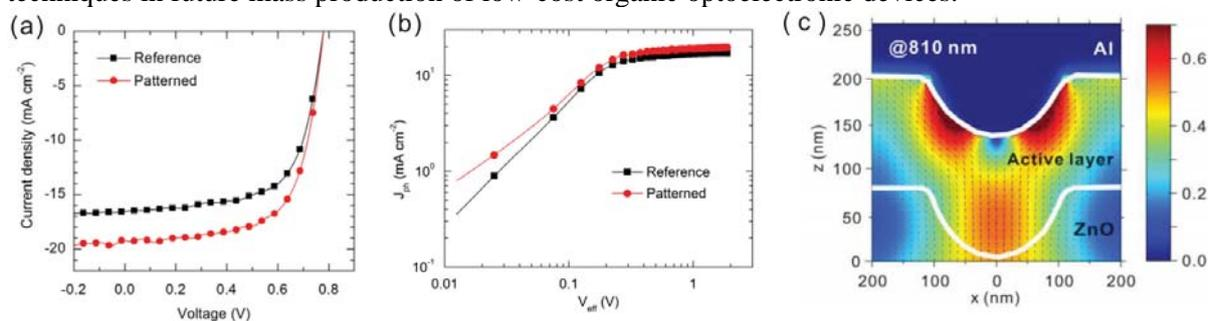
**Figure.** Device performance of polymer solar cells with and without light trapping Scheme.
